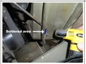
Your radiator overflow tubing is soldered to the shroud in a couple places. We need to remove one of them in order to prepare connection to the desert cooling tubing. By holding a micro-torch to the soldered area for a few seconds, wedge a screwdriver into this area apply pressure to pop off.
