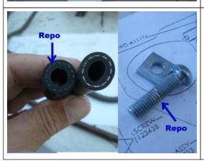
Another issue discovered with the Repo kit was the hose size...which was smaller than we would hoped for the clamps (so we replaced with better), AND the clamp screws stripped really easily when tightening down. So we replaced with NOS 10-24's.
