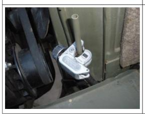
Use a small tubing cutter to cut the radiator overflow line, and the desert cooling line. Here we show an example, but easier if you take the tubing out of the area.
