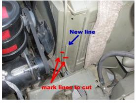
surge tank. Here we want to measure it up and see how it will line up to the radiator hose. Next, remove your battery, hold the surge tank up against the grill with the new line running through the second grill opening on the passenger side. Run the line under
